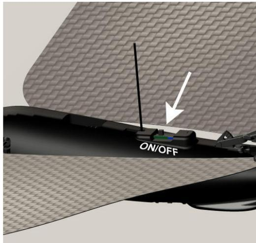
**Detecting the bird:** Launch the application (or click on “FIND BIRD” in the NEST), and turn on the bird. The “scanning bird” screen above will appear. The bird will be detected immediately.
