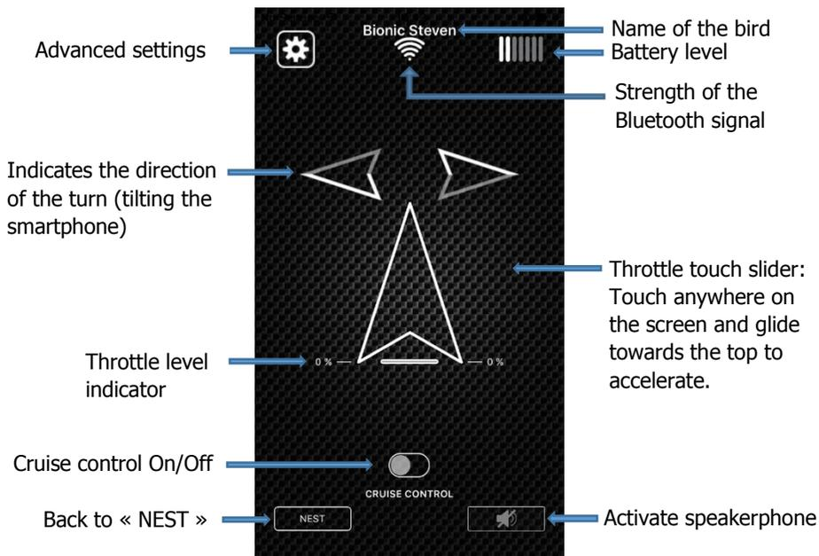
**Direction:** The direction of a turn (right/left) and its angle is controlled by the tilt angle of the smartphone. The arrow becomes progressively grey when the tilting is active. Tilt sensitivity can be altered in the advanced settings screen.
