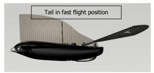
\* For outdoor flights, in a big space or for fast flights: adjust the tail in a low position (using the notch 1 or 2).
