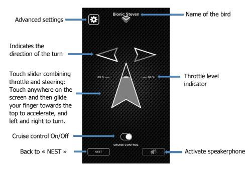
By placing your index finger on the screen, you define the zero position of the throttle/steering cursor.
