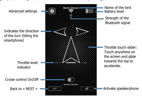
Direction: The direction of a turn (right/left) and its angle is controlled by the tilt angle of the smartphone. The arrow becomes progressively grey when the tilting is active. Tilt sensitivity can be altered in the advanced settings screen.
