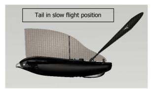
\* For indoor flights, in a confined space, or for slow flights: set the tail in a high position (choose the notch n° 3, starting from the bottom, among the 5 possible positions). The notches 4 and 5 are not recommended at begin.
