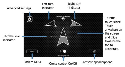
Typically, for a right-handed person, the right thumb guides the speed while the hands turn the smartphone like a steering wheel to steer the bird.
