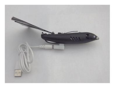
To charge BIONIC BIRD, simply connect the magnetic contact points located under the bird's body and the top of the plug adapter as shown on the picture. They magnetically connect to each other automatically and the bird will sit firmly on it. Then connect the cable to your smartphone charger or to a USB socket of your computer.
