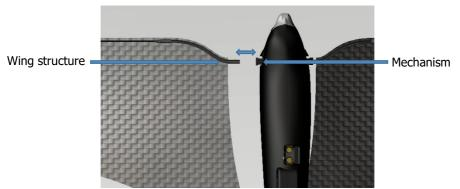
Then detach the front of the wing: hold the wing structure firmly and pull it out so that it comes out the slot. It is not necessary to change both wings, when just one is broken. Choose the appropriate spare wing (left or right) corresponding to the one to be replaced. Proceed reverse way: Start by inserting the wing structure in the slot, you should feel a "click" which means that the wing is correctly inserted.
