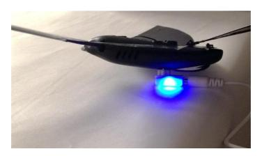
The upper part of the adapter lights in red when it starts to charge. Charging takes around 18 minutes. When BIONIC BIRD is fully charged and ready to fly again, light turn in blue. Note: - The light can be difficult to see when outdoors in direct sunlight. It's easiest to check the light in a shadow to see whether BIONIC BIRD is charged.
