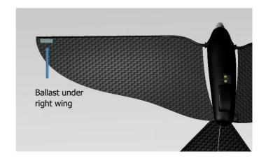
If the bird tends to turn to the left, add some weight to the right wing: Take one of the aluminium tape piece and stick it near the tip of the right wing, below the wing, as shown on the picture.
