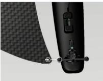
1 – At rear, snap the back of the wing on the round knob of the steering mechanism.
