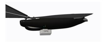
To charge MetaBird, simply insert MetaBird's connectors into the charging slot of the adapter. Then connect the cable to your smartphone charger or to a USB socket of your computer.
